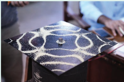
Visualization of a standing wave pattern in a Chladni plate
