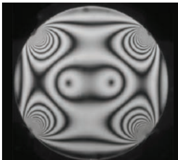
Photoelastic visualization of stresses in a roller bearing under peripheral loading.
