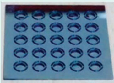
An array of cricket inspired MEMS speakers fabricated on a "Silicon on Insulator" wafer.
