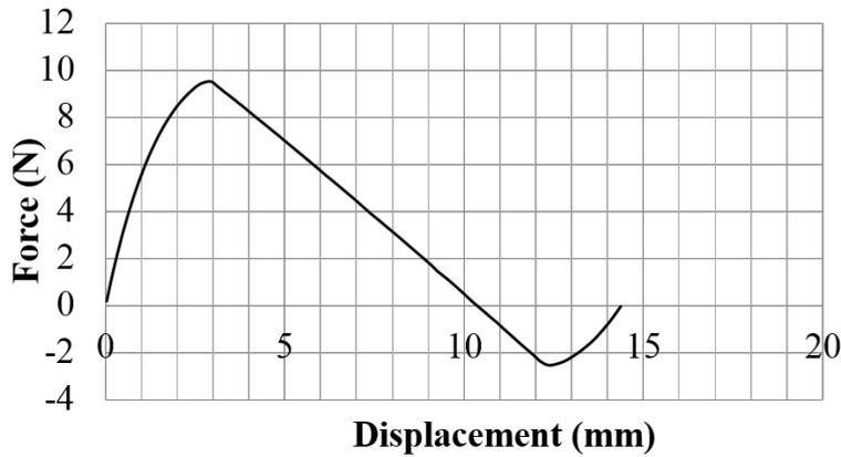
Figure 6.14: Force-displacement curve for actuation at the mid-point of the input arches 1 and 2
