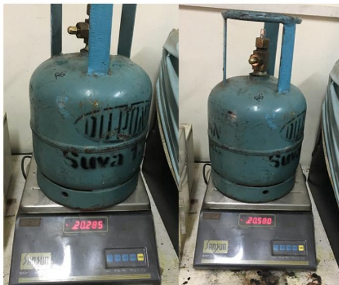
Figure 4.25: Refrigerant bottle and weigh balance device.
