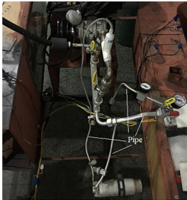
Figure 4.11: Aluminium pipes and fittings.
