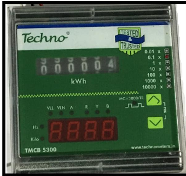
Figure 4.21: Three phase energy meter.
