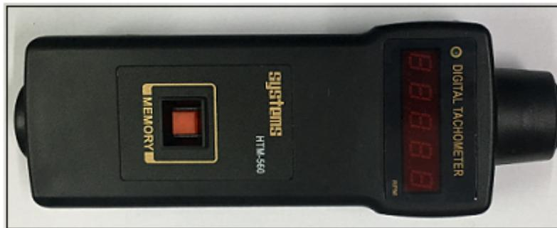
Figure 4.20: Digital tachometer.
