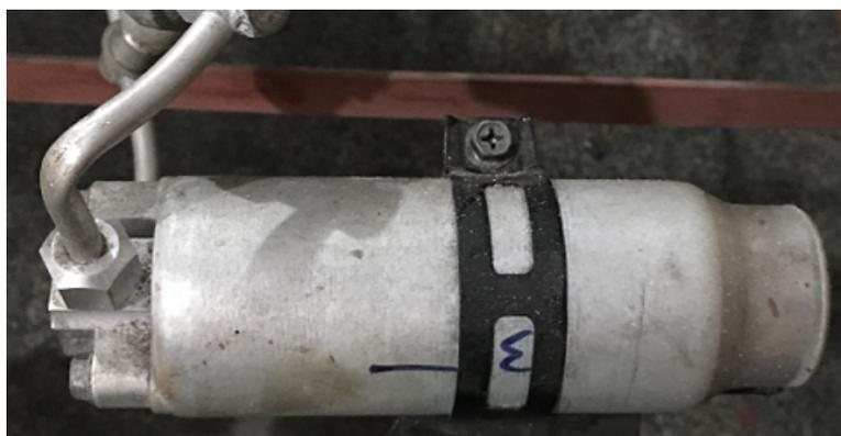
Figure 4.10: Receiver or Dryer
