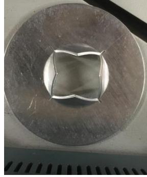
Fig. 4.2: Burst diaphragm after the test
