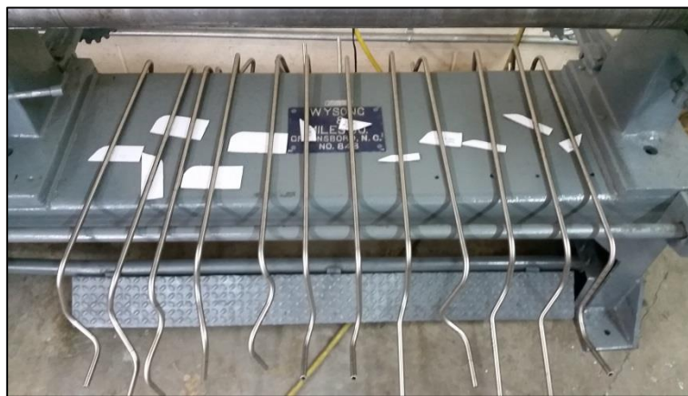
Fig. 6.7: Tubes needed for the back panels, bent by Albina, Inc
