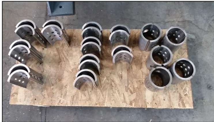
Fig. 6.6: Headers cut by Springs Fabrication
