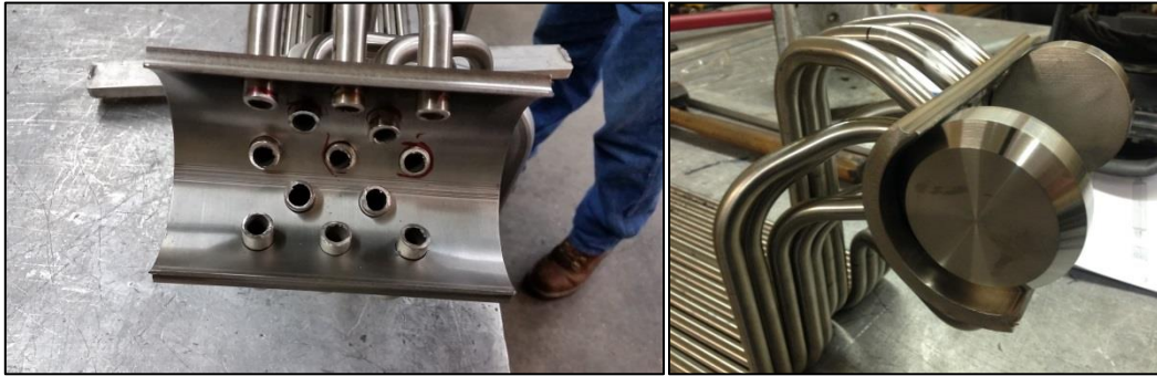
Fig. 6.8: Header with inserted tubes and header caps in place before welding
