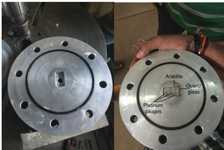
Fig. 4.4: End-flange with cavity for mounting sensor and assembled flange
