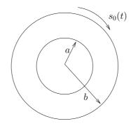
Figure 1: Hollow disk fixed rigidly at the inner boundary r = a, and subjected to tangential tractions  $s_0(t)$  on the outer boundary r = b.
