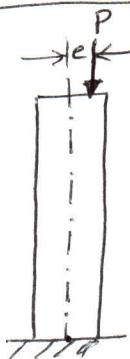
If the load is eccentric, i.e. if it acts slightly off from the neutral axis, the critical load reduces because the moment due to the eccentric load tends to bend the column for a much smaller  $P$ .
