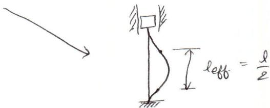
we consider that a column has failed if it buckles or if it gets crushed (or yielding) under compressive loading when  $|\sigma_c|$  exceeds  $\sigma_y$ . A short column fails by getting crushed (or yielding) and a long column fails by buckling. We define a slenderness ratio to characterize a column as short or long.
