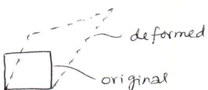
stores both hydrostatic strain energy and distortion energy
