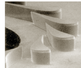
Detail of the DRIE-etched blades
