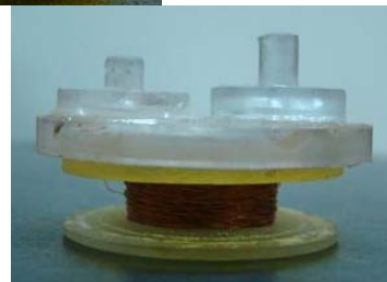
Wound coils and assembly
