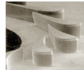
Detail of the DRIE-etched blades
