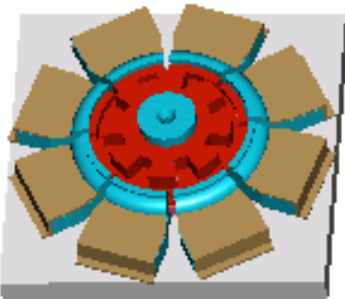
Deposit and etch metal
