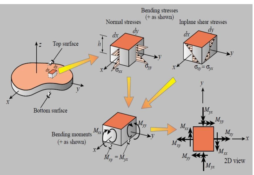
• According to hook's law for plane stress, (so no shear forces)[5]
