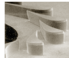
Detail of the DRIE-etched blades
