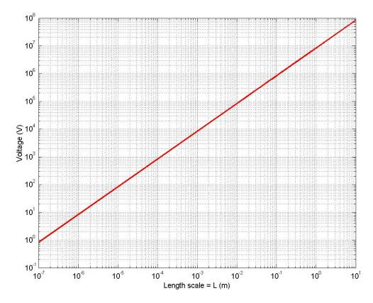
The equation used to plot the above graph makes it clear that the required voltage to get the same fraction of deflection increases linearly with the length scale. So, it is impractical to get substantive deflection with electrostatic force at larger length scales. On the other hand, at the MEMS scale and below, it is quite attractive.
