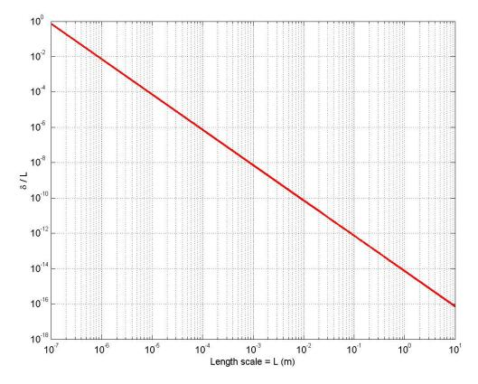
It is clear from this plot and the equation above that the ratio of the maximum beam deflection to the length of the beam, at a given voltage, decreases rapidly with increasing length scale. Hence, the electrostatic force is favorable at small length scales.
