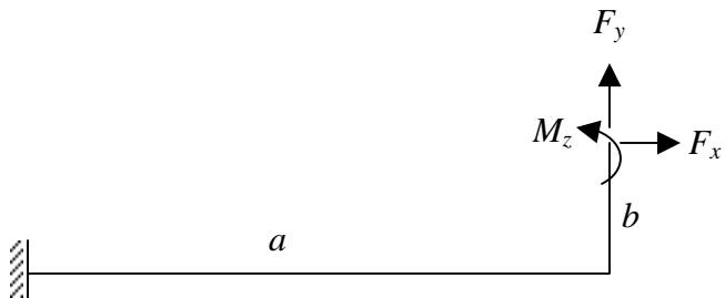
We consider vertical and horizontal forces and the moment at the end because we need to solve for the end being guided in x and y directions.
