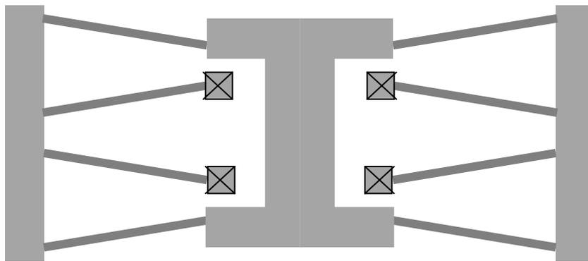
11. Partially de-coupled XY suspension
