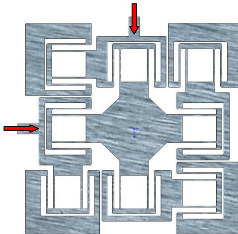
13. Two-layer fully de-coupled XY suspension with amplification
