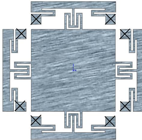
12. Fully de-coupled XY suspension
