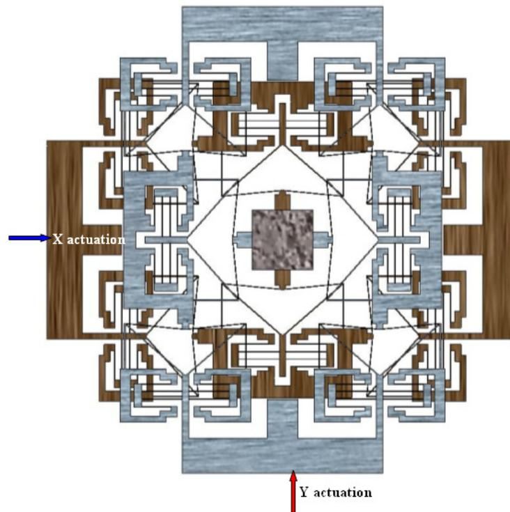
14. Left symmetric half of a single-layer fully de-coupled XY suspension with amplification
