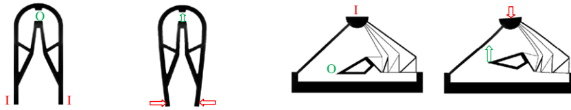
Fig. 1. Compliant mechanisms in original and deformed configurations with input (I) and output (O) ports marked.
