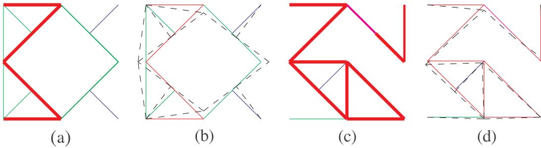
**Fig. 5** A synthesis example of a displacement inverter using sequential quadratic programming. (a) Optimal topology I of displacement inverter, (b) deformed profile, (c) optimal topology II of displacement inverter obtained using asymmetric initial guess, (d) deformed profile
