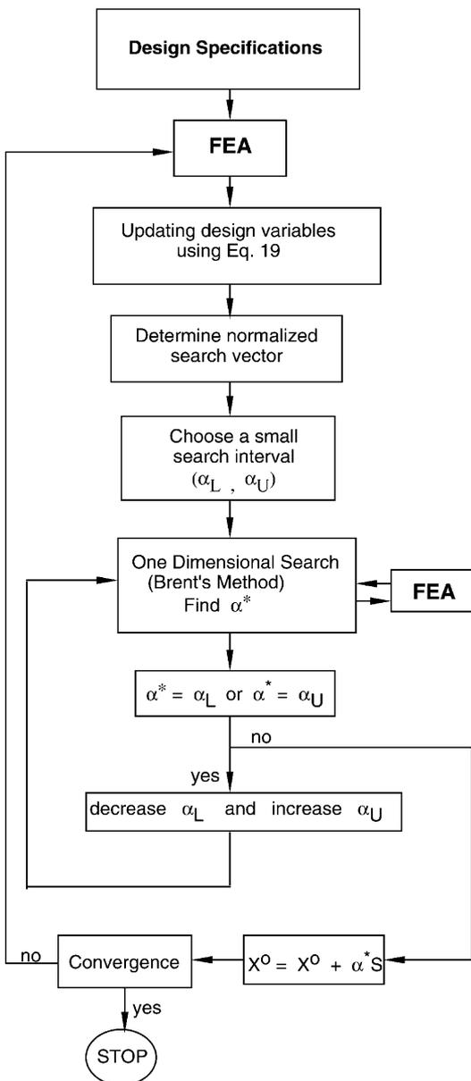
**Fig. 6** Schematic of the optimality criteria approach
