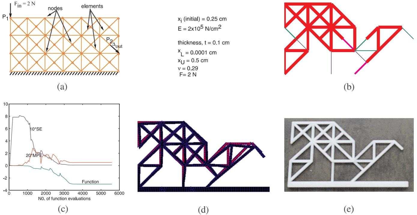
**Fig. 7** Synthesis example of a compliant pliers using formulation (P2). (a) Problem specification on the ground structure, (b) optimal topology, (c) convergence history, (d) finite element analysis with plane stress elements, (e) realized modified mechanism manufactured using ABS plastic
