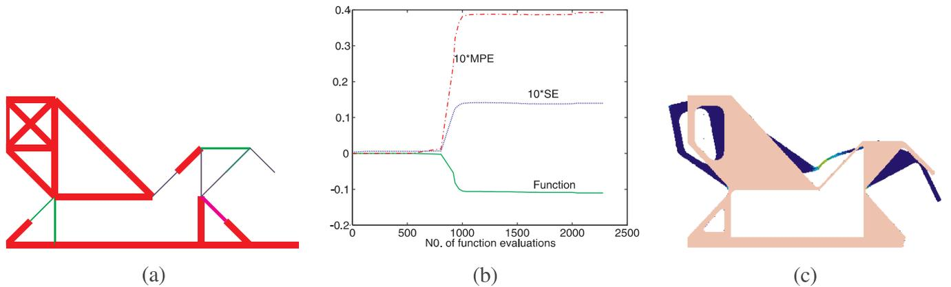
**Fig. 8** Synthesis of a compliant pliers using the energy based objective. (a) Optimal topology, (b) convergence history, (c) finite element analysis with plane stress elements
