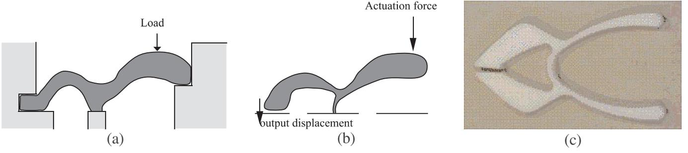
**Fig. 1** (a) A structure, (b) symmetric half of the compliant mechanism shown in (c)
