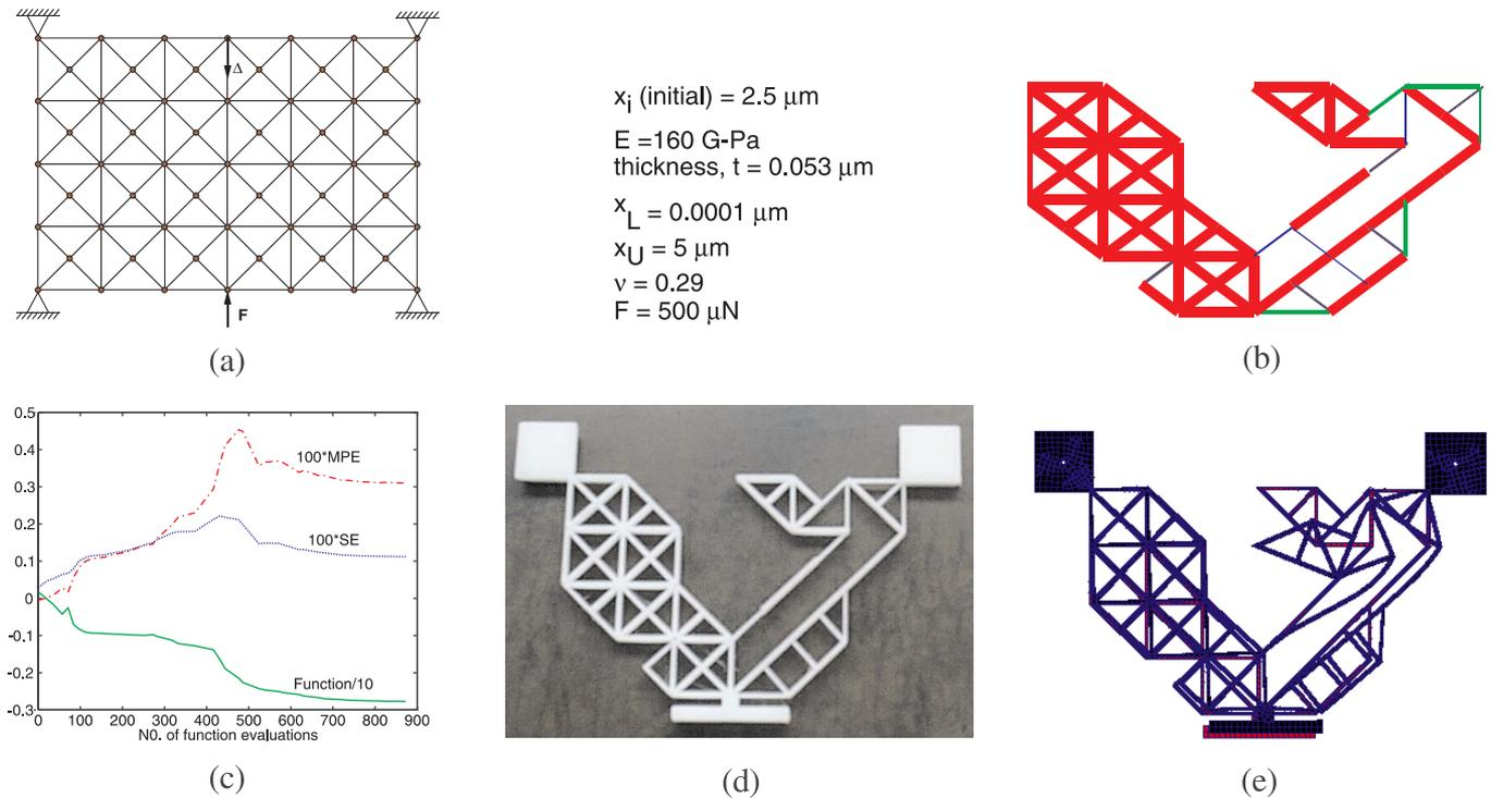
**Fig. 10** Synthesis example of micro compliant amplifier. (a) Problem specification on the ground structure, (b) optimal topology (obtained using asymmetric initial guess), (c) convergence history, (d) realized design with ABS plastic, (e) finite element analysis with plane stress elements
