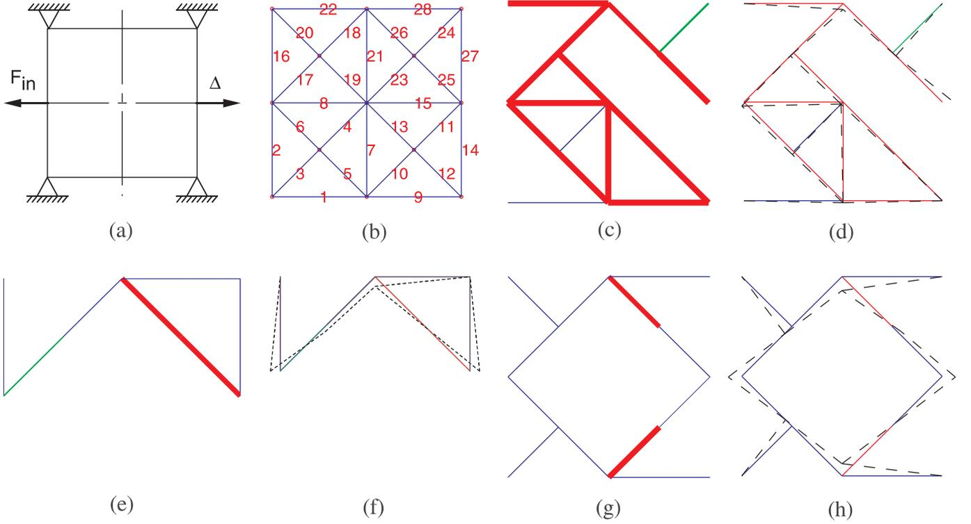
**Fig. 3** A synthesis example of the displacement inverter using sequential quadratic programming. (a) Design domain for compliant inverter, (b) a frame elements mesh, (c)–(d) optimal topology of displacement inverter for  $-\frac{MPE}{SE}$  and the deformed profile, (e)–(f) optimal topology and deformed profile for  $-\text{sign}(MPE)\frac{MPE^2}{SE}$ , (g)–(h) optimal topology and deformed configuration for  $-\frac{MPE}{e^{SE}}$
