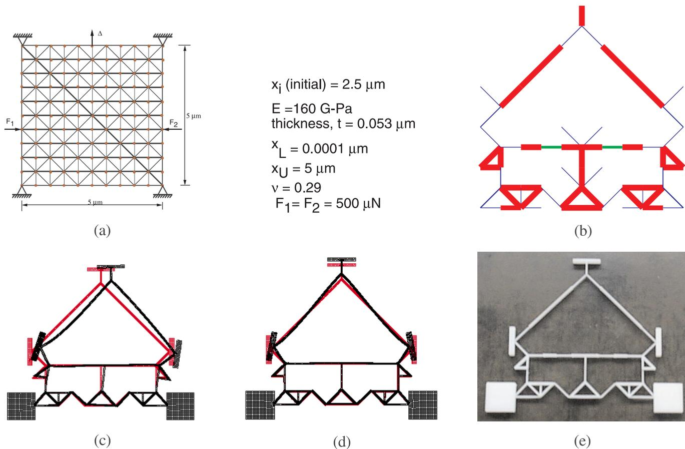
**Fig. 11** Synthesis example of a micro **AND** logic gate. (a) Design specifications, (b) optimal topology of the AND gate, (c) deformed configuration with a single load, (d) deformed configuration with both loads, (e) prototype of the AND gate fabricated with the ABS plastic
