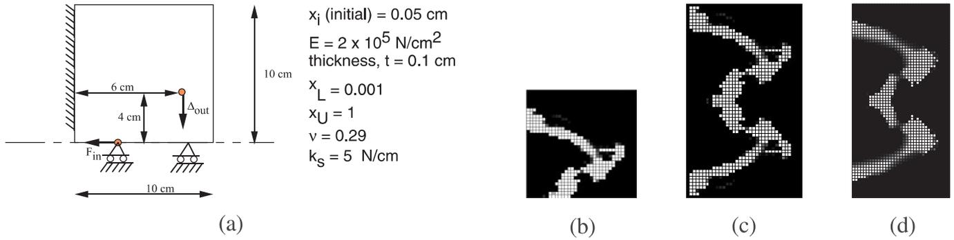
**Fig. 9** Synthesis of compliant grippers using bilinear plane stress elements. (a) Design domain for the symmetric half, (b) optimal topology for the symmetric half of compliant grippers using formulation (P2), (c) optimal topology for compliant grippers, (d) optimal topology for grippers using the energy based approach of formulation (P3)
