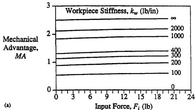
Fig. 5 (a) Type 3 mechanical advantage plot
