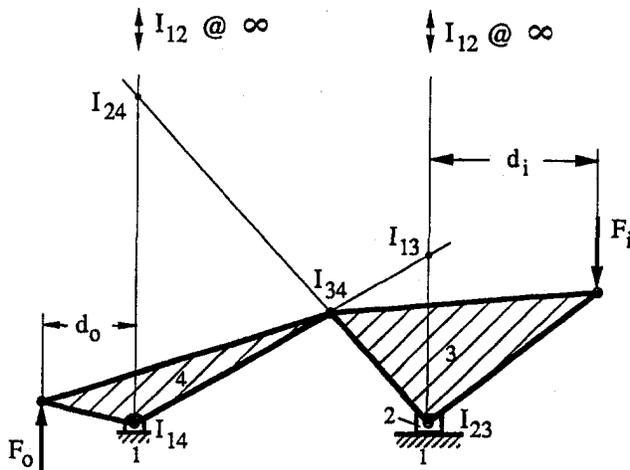
Fig. 1 Rigid-body slider crank mechanism
