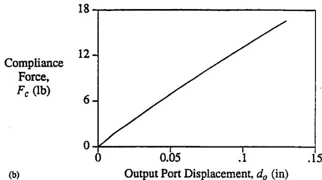
Fig. 3 (b) Compliance force ( $F_c$ ) variation with output port displacement ( $d_o$ )
