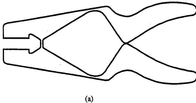
Fig. 2 (a) A compliant crimping mechanism
