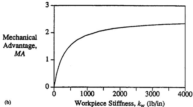
Fig. 5 (b) Mechanical advantage variation with workpiece stiffness
