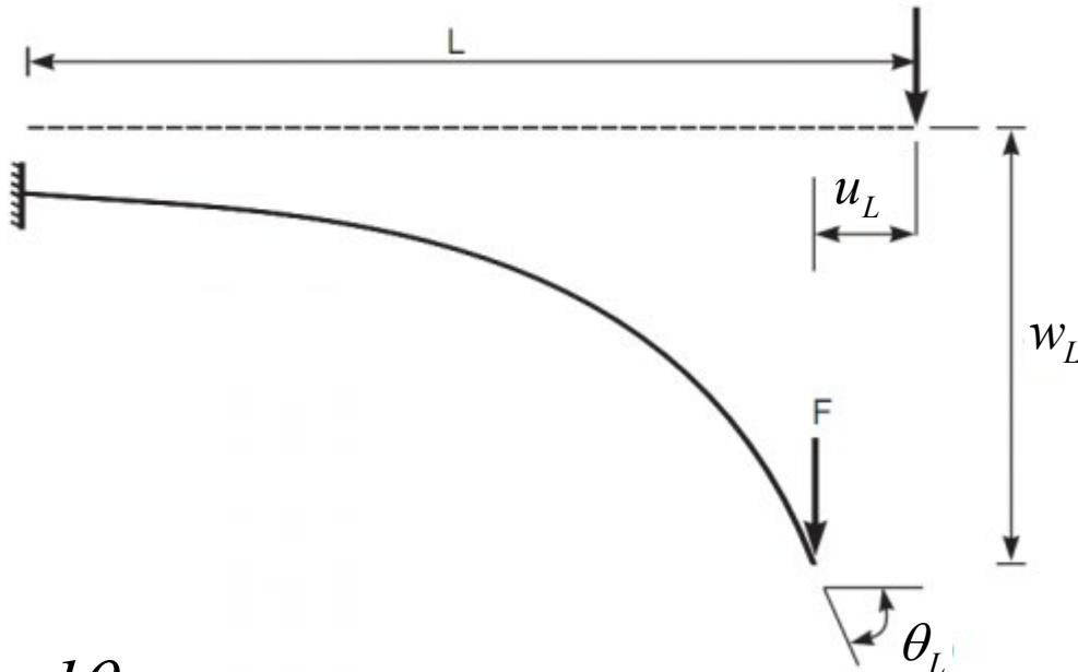
$$EI \frac{d\theta}{ds} = F(L - x - u_L) \quad \text{Large displacements}$$
