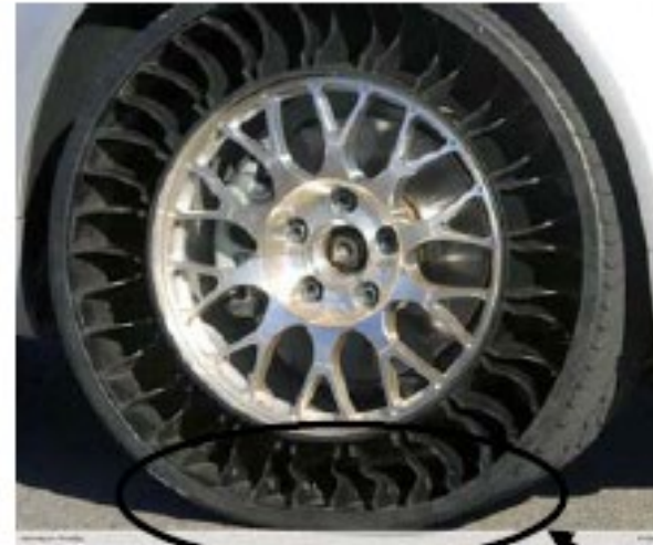
Flattening of tire under loading in tweel , an experimental design made by michelin and inspiration for this project
