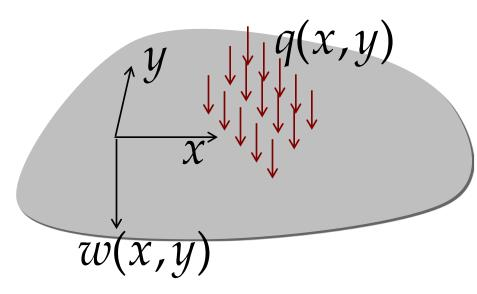
A plate subjected to a transverse load q(x,y). Its deformation w(x,y) can be determined by minimizing the potential energy.
