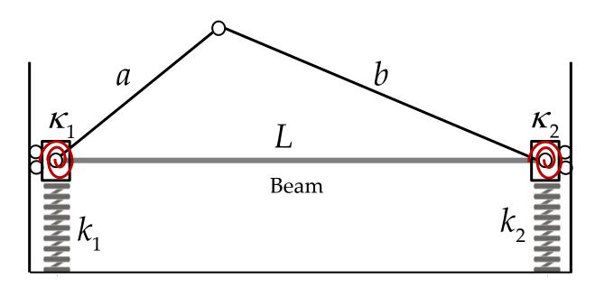
Here, the transverse displacements and rotations at the two ends are coupled to one another because of the asymmetric linkage that connects them. We need to write the strain energy and then take Gâteaux variation.
