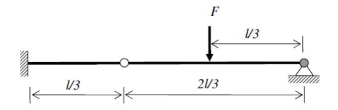
Four boundary conditions are obtained when we minimize the potential energy of a beam under transverse load. Think of a physical arrangement of a beam where two or more boundary conditions are coupled to one another so that the four boundary conditions are not all independently zero. Sketch your physical arrangement clearly and mathematically interpret how the boundary conditions are coupled.
