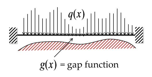
Calculus of variations problem, in the framework of minimum potential energy principle, can easily account for contact conditions, as shown here. Just an inequality constraint!
