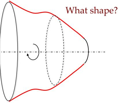
Given end points  $(x_1, y_1)$  and  $(x_2, y_2)$ , find the curve which when rotated about the *x*-axis will have least surface of revolution.
