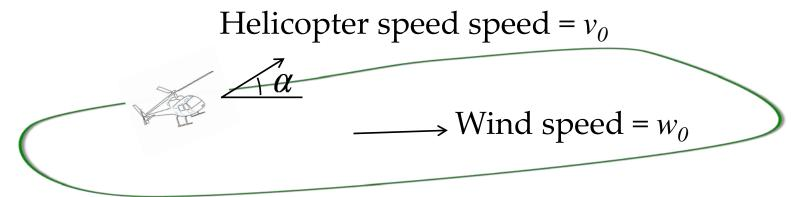
A surveillance helicopter travelling at constant speed ( $v_o$ ) under the constant wind speed of ( $w_o$ ) needs to enclose maximum area by taking a closed path in a given time T. The optimization variable is the steering angle,  $\alpha(t)$ . The starting point is ( $x_o, y_o$ ).
