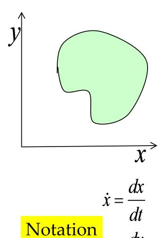
It is convenient to use parametric representation of a closed curve because explicit form y(x) may need to be multivalued. Let t = 0 to L, be the parameter. Let the curve be given by x(t) and y(t).
