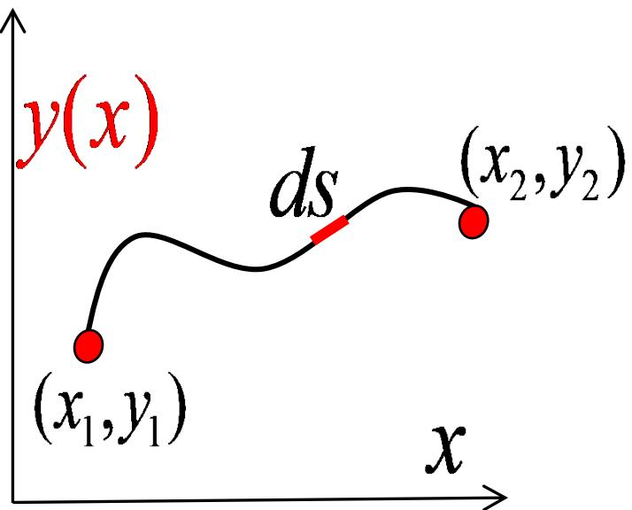
$$\underset{y(x)}{\text{Min}} \ L = \int_{x_1}^{x_2} \sqrt{1+y'^2} \ dx$$
