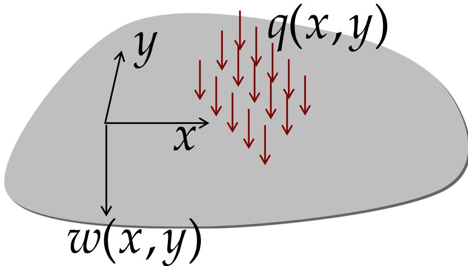
A plate subjected to a transverse load  $q(x, y)$ . Its deformation  $w(x, y)$  can be determined by minimizing the potential energy.
