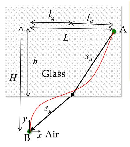
$$\underset{y(x)}{\text{Min}} T = \int_{0}^{L} \left( \frac{\sqrt{1 + {y'}^{2}}}{v(y)} \right) dx \\
