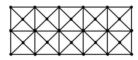
If optimized values of "b"s reach the lower bound (which is nearly zero), then the corresponding beams elements "disappear" in the design leaving the optimized topology.
