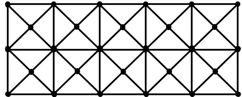
If optimized values of “b”s reach the lower bound (which is nearly zero), then the corresponding beams elements “disappear” in the design leaving the optimized topology.
