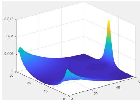
4 Level-set plane moves in the topological sensitivity field, such that the volume constraint is satisfied.
