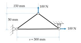
(b) Now, pose and solve the same problem as a shape optimization problem in one variable wherein the location of the moving pivot is variable from the fixed pivot. That is, 300 mm (call it s) can be varied and its optimum value needs to be found. Plot strain energy and volume as functions of s and verify that the optimum you found is indeed so.
