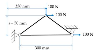
(b) Now, pose and solve the same problem as a shape optimization problem in one variable wherein the height of the truss is variable. That is, 50 mm (call it s) can be varied and its optimum value needs to be found. Plot the strain energy and volume as functions of s and verify that the optimum you found is indeed so.
