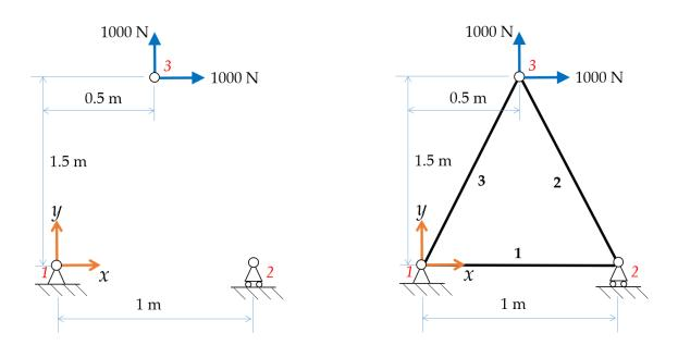
On the left side, we see that three points are shown. Point 1 is fixed. Point 2 can move the x direction but it is fixed in the y direction. Point 3 has two external forces. On the right side, we see a three-bar truss. It has a particular topology (one hole) with a certain shape. If we move a point in a given topology, we get a differently shaped truss.
