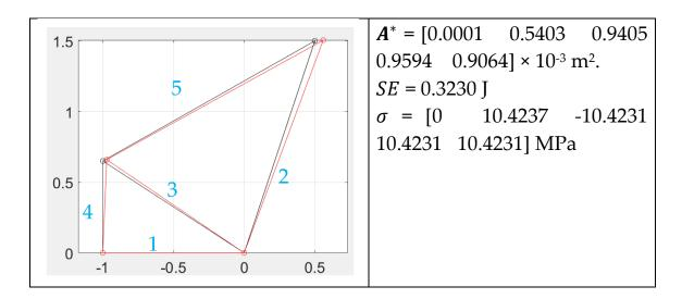
So, if we vary the *x* coordinate of vertex 3 and find an optimum value, we can find the best shape of the truss.
