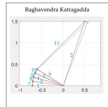
$A^* = [0.0110 \quad 0.0000 \quad 0.0222$   $0.0222 \quad 0.0222 \quad 0.0488 \quad 0.1604$  $0.1604 \quad 0.1604 \quad 0.1644] \times 10^{-3} \text{ m}^2.$
