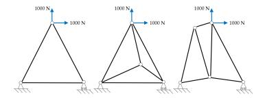
Now, we can change the shape of each topology to get differently shaped trusses for that topology. And then, when we vary the areas of cross-section of the truss members, we get different response of the truss for the applied external loads.
