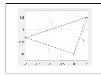
$A^* = [0.0658 \quad 0.0658] \times 10^{-3}$   $m^2$ . SE = 0.4290 J  $\sigma = [-12.0126 \quad 12.0126]$  MPa
