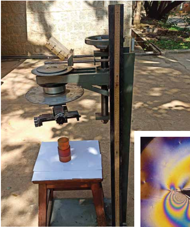
Left: The Scattered Light Polariscope designed by Prof LS Srinath. Right: Scattered fringes as seen in the polariscope
