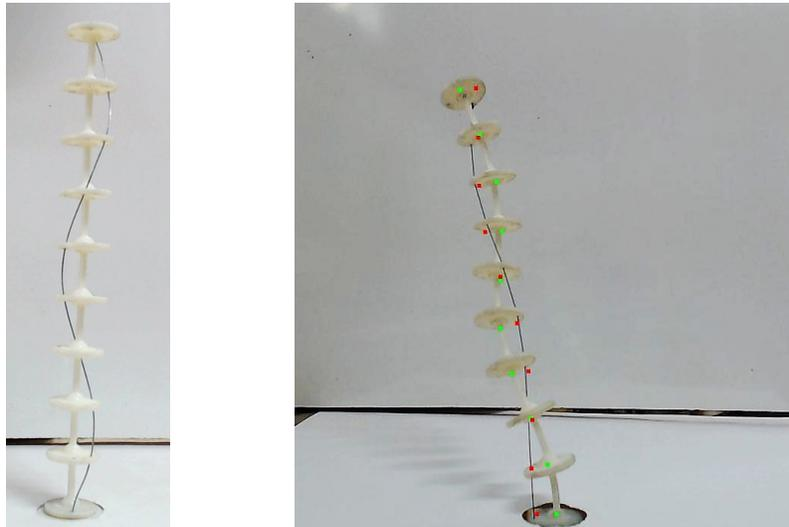
Fig. 11: Initial and actuated configurations of a continuum robot with  $\phi_i = 60^\circ, i = 1, 2, \dots, 9$
