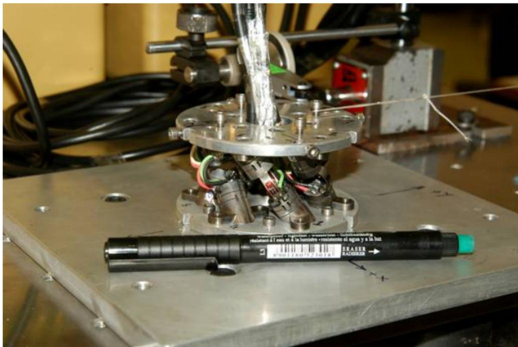
**Figure 44:** Prototype sensor sensitive to moment components
