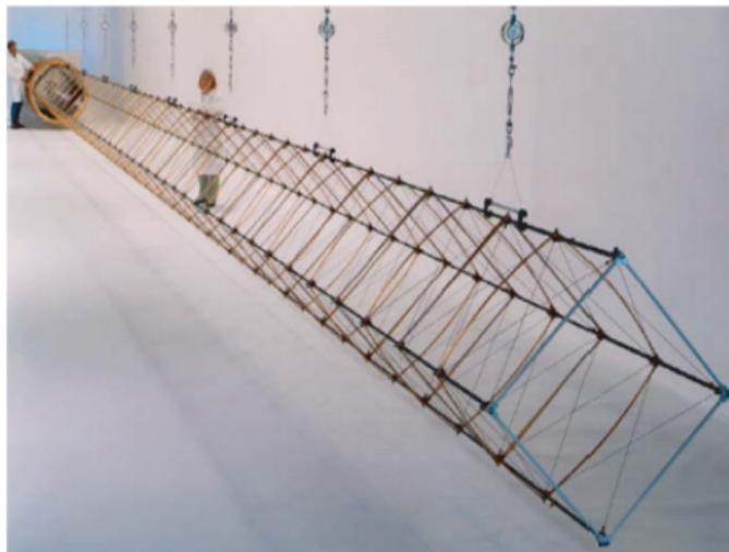
**Figure 45:** Folded articulated square mast (FAST)
