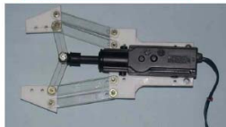
A four-bar mechanism to move gripper jaws
