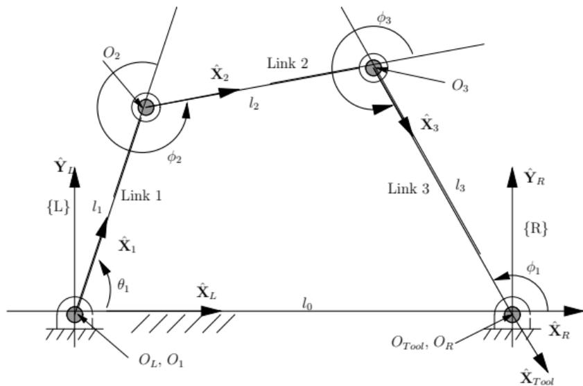
Figure 2: The four-bar mechanism
