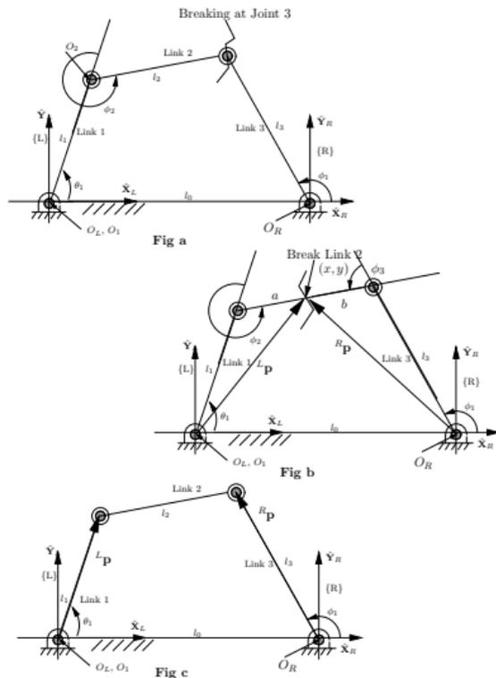
Figure 4: The four-bar mechanism 'broken' in different ways
