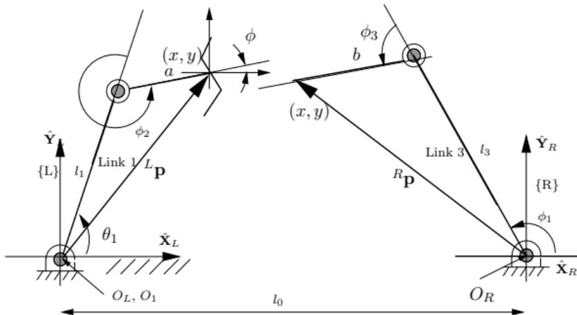
**Figure 10:** Inverse kinematics of a four-bar mechanism
