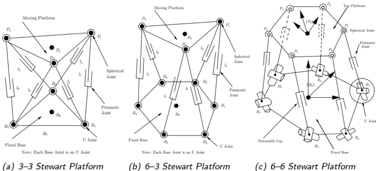
Figure 13: Three configurations of Stewart platform manipulator
