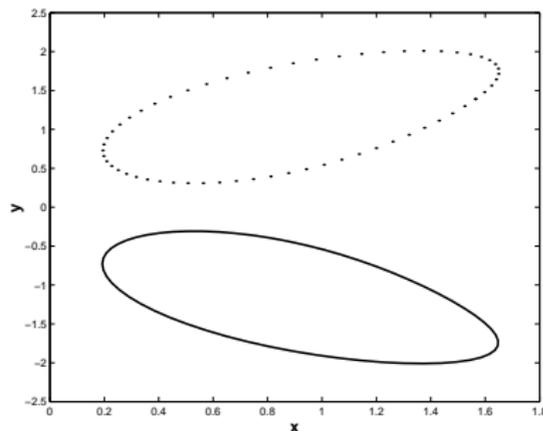
(b) Coupler curves for 4-bar mechanism
