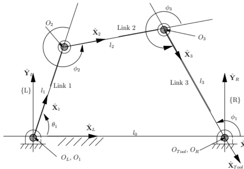
**Figure 5:** The four-bar mechanism - revisited
