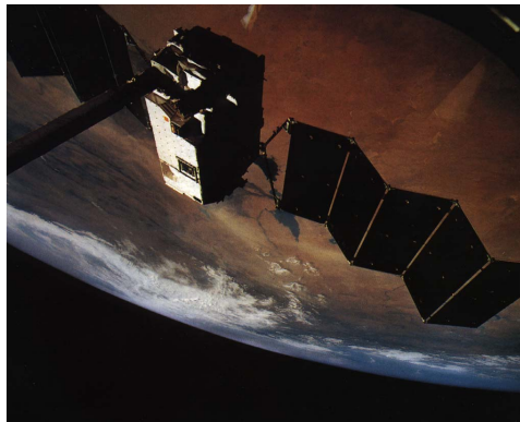
Figure 3: Solar panels being deployed
