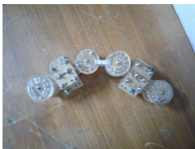
Figure 3: Two rigid spine segment connected by a flexible strip
