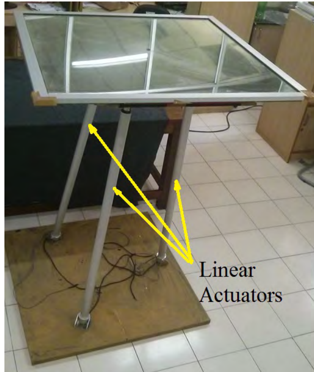
Fig. 12: Prototype of 3-RPS heliostat
