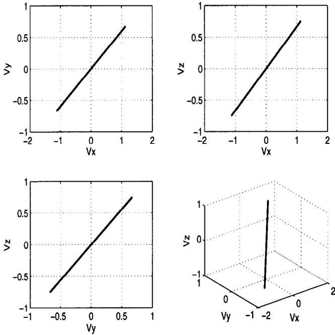
Figure 3. Degenerate velocity "ellipse" at a singular point
