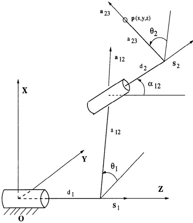
Figure 1. A schematic of a general 2R manipulator
