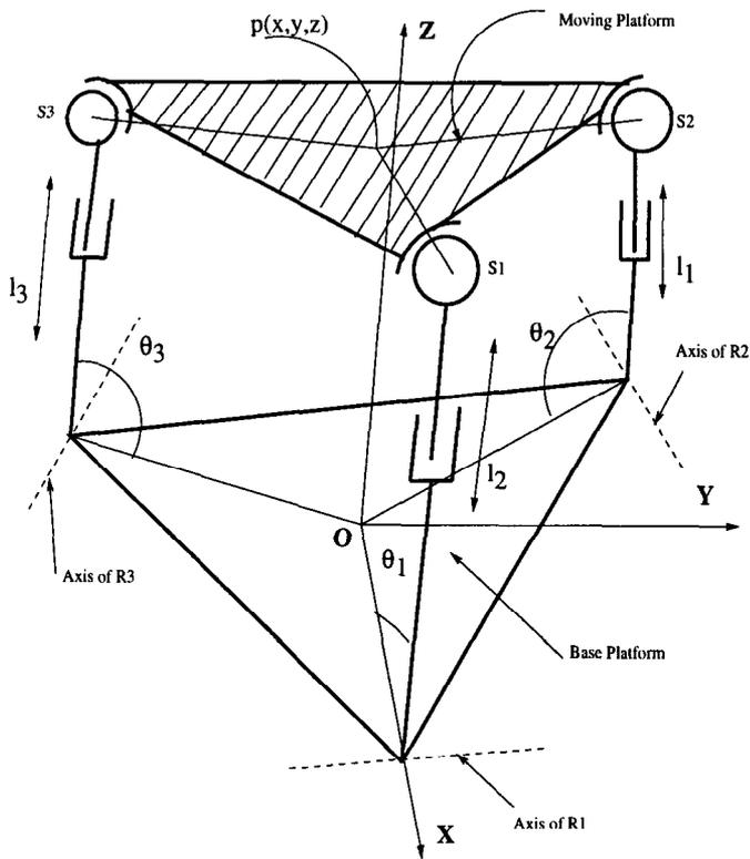
Figure 4. The RPSSPR-SPR parallel manipulator
