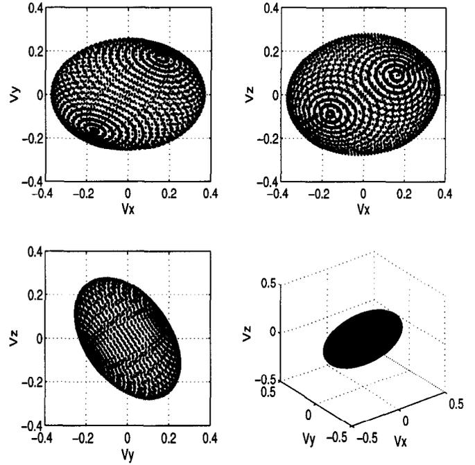
Figure 5. Velocity ellipsoid at a non-singular point
