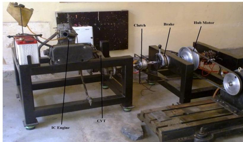
Figure 2: Experimental setup for low cost hybrid propulsion with speed addition
