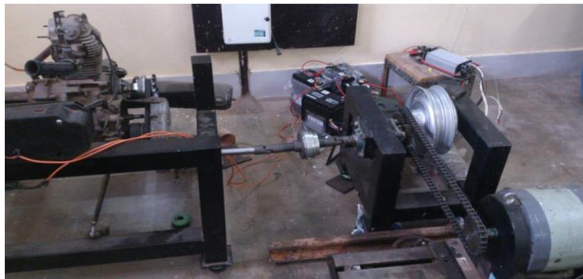
Figure 3: Experimental setup for low cost hybrid propulsion with torque addition
