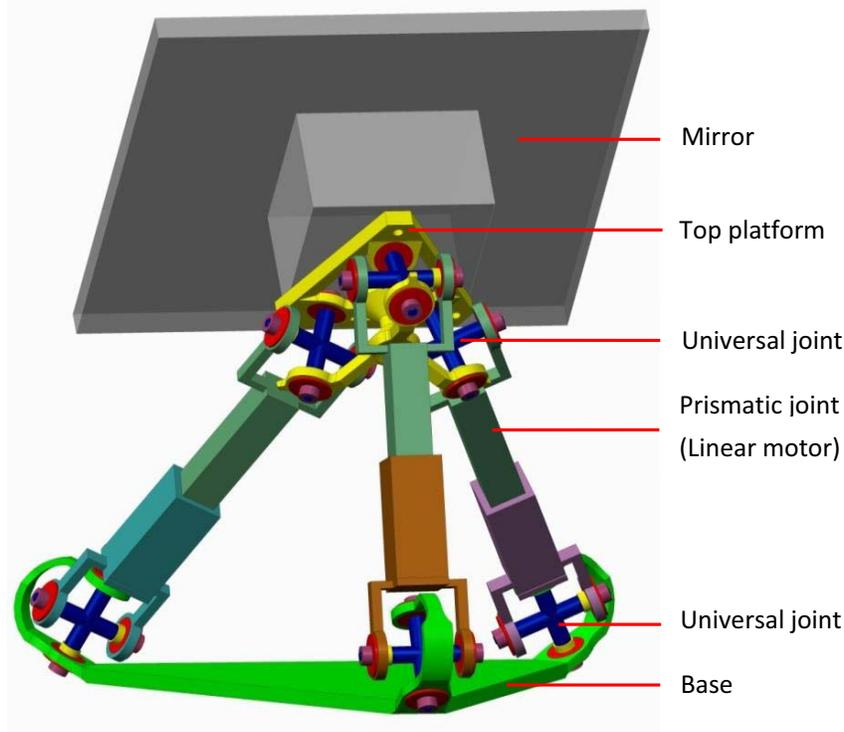
Figure 1: A solid (CAD) model of a parallel 3-UPU-wrist manipulator.
