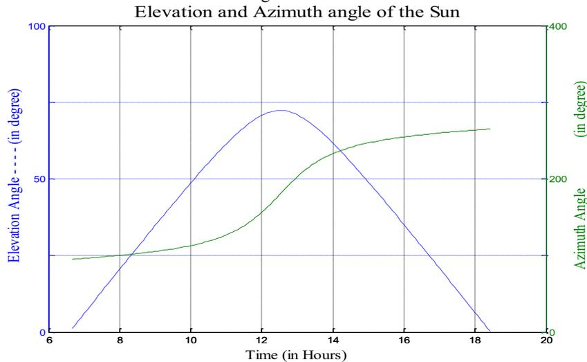
Figure 3: Plot of Azimuth and Elevation angle of Sun on 8<sup>th</sup> March 2015 at 12°58'13" latitude and 77°33'37" longitude
