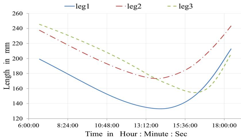
Figure 4: Plot of prismatic joints vs. time in GMT for  $12^\circ 58' 13''$  latitude and  $77^\circ 33' 37''$  longitude on 8<sup>th</sup> March 2015.
