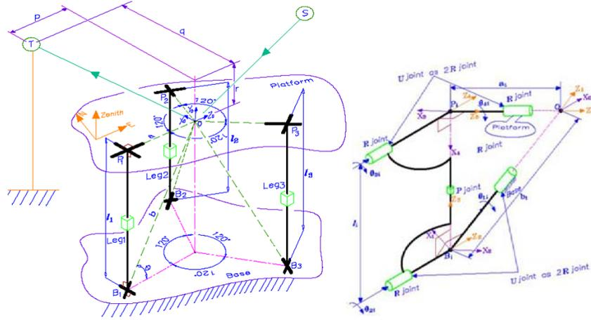
Figure 2: Schematic representation of a 3-UPU spherical wrist manipulator and the 'i'th leg, made using AutoCAD [10].
