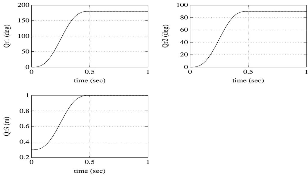
Figure 4: Desired and actual joint position trajectory
