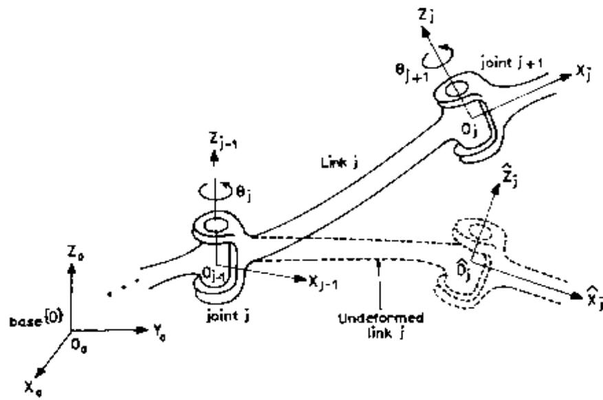
Figure 1: Coordinate systems for the flexible link  $j$
