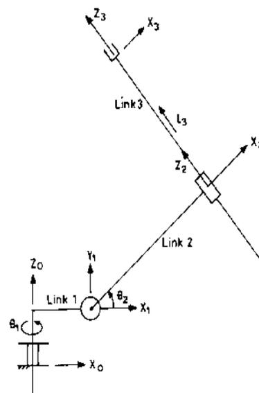
Figure 3: Flexible spherical (RRP) manipulator
