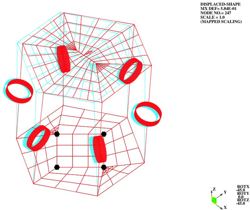
Figure 12: Deflection (mm) of the sensor
