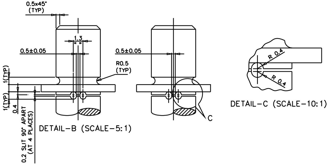
Figure 11: Detailed view of the flexural hinge
