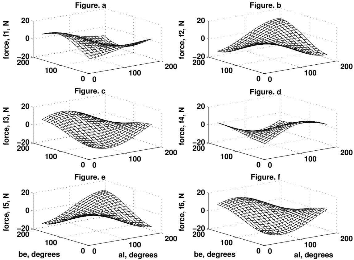
Figure 8: Leg forces versus 'al' and 'be' - only forces applied
