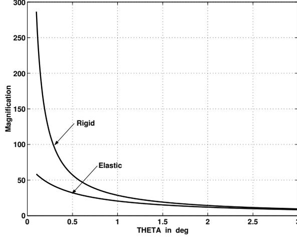
Figure 2: Magnification in axial force in the link as a function of  $\theta$
