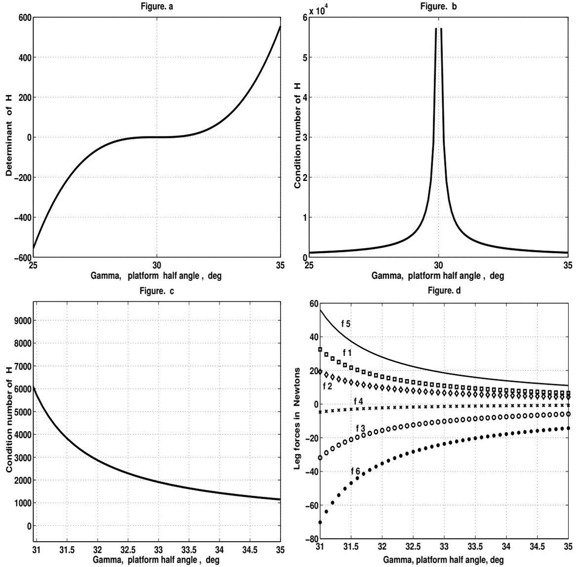
Figure 6: Plot of  $\det[H]$ , Condition No. of  $[H]$  and Leg forces with  $\gamma$
