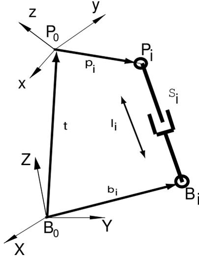
Figure 5: A typical leg of a 6 – 6 Stewart Platform
