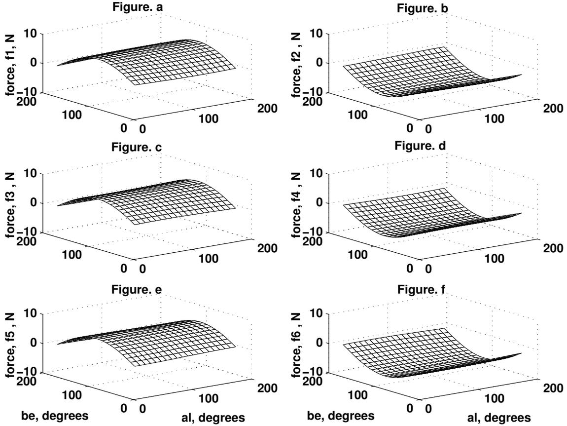
Figure 9: Leg forces versus ‘al’ and ‘be’ - only moments applied
