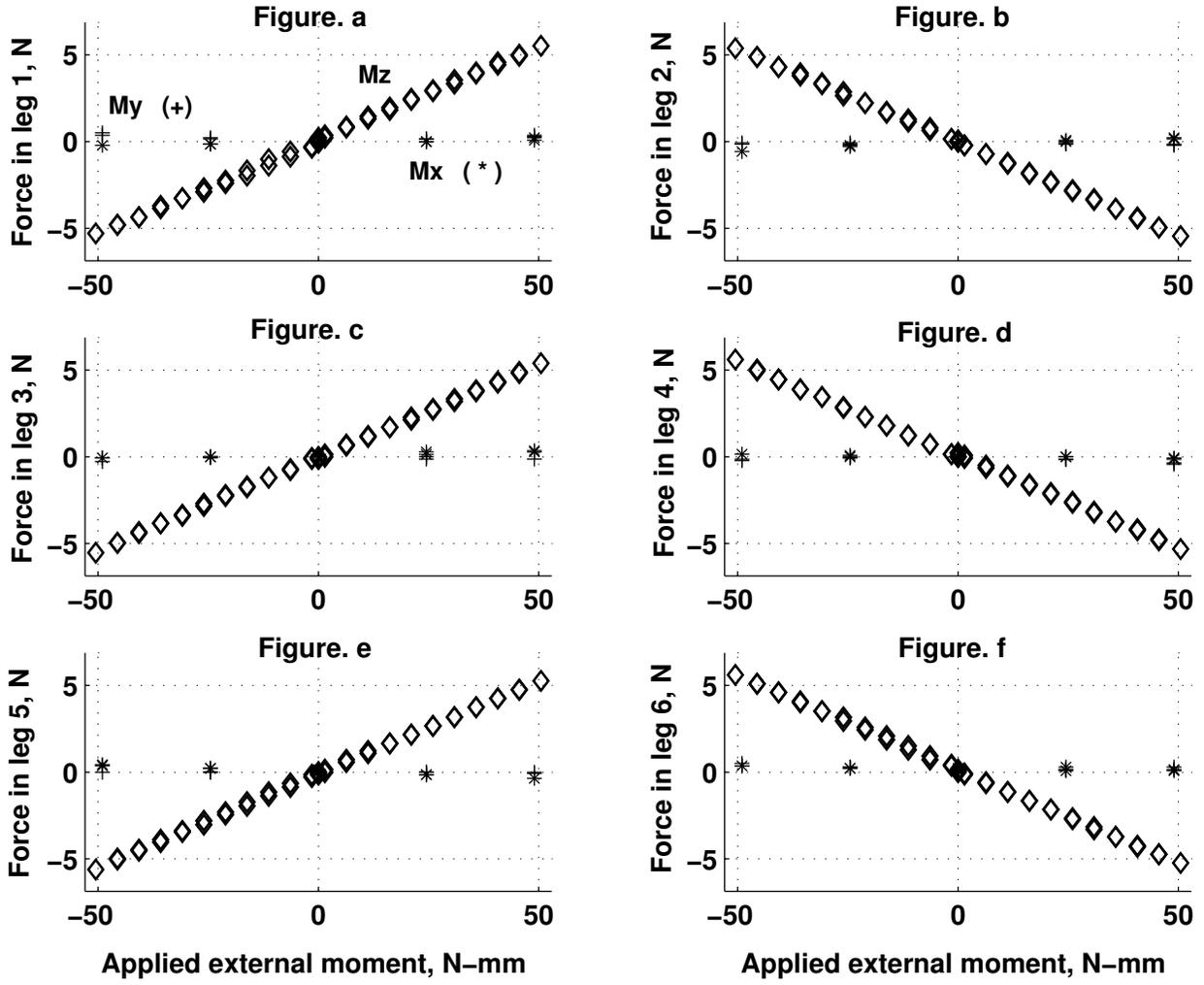
Figure 16: Experimental data for applied external moment
