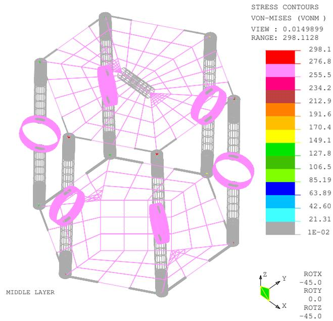
Figure 13: Stress (N/mm<sup>2</sup>) in the sensor
