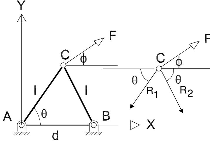
Figure 1: A planar two link hinged truss
