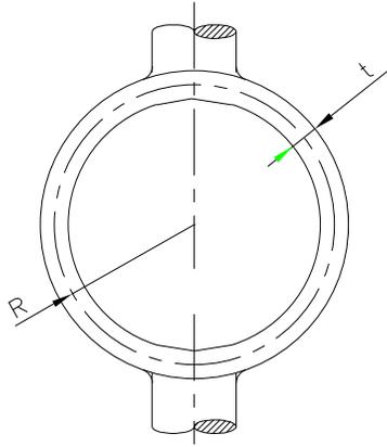
Figure 10: Schematic of the sensing element
