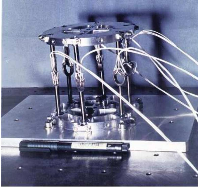
Figure 14: Stewart platform based force-torque sensor
