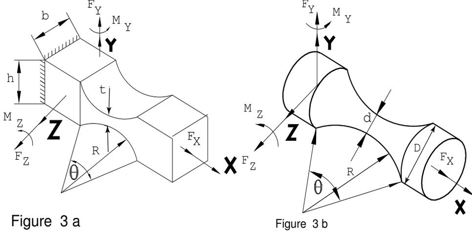
Figure 3: Flexure hinges
