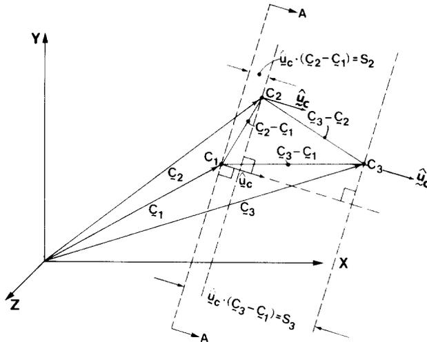
Fig. 6. The three positions of the  $C-S$  link and the associated vectors.
