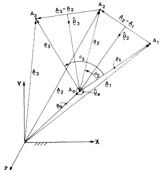
Fig. 4. The three positions of the  $R$ - $S$  link  $\mathbf{a}$  and the associated vectors.
