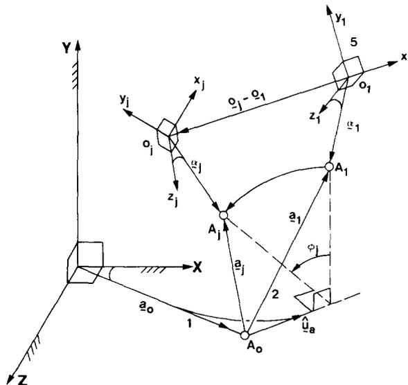
Fig. 3. Schematic of the 1st and the  $j$ th positions of links 2 and 5.
