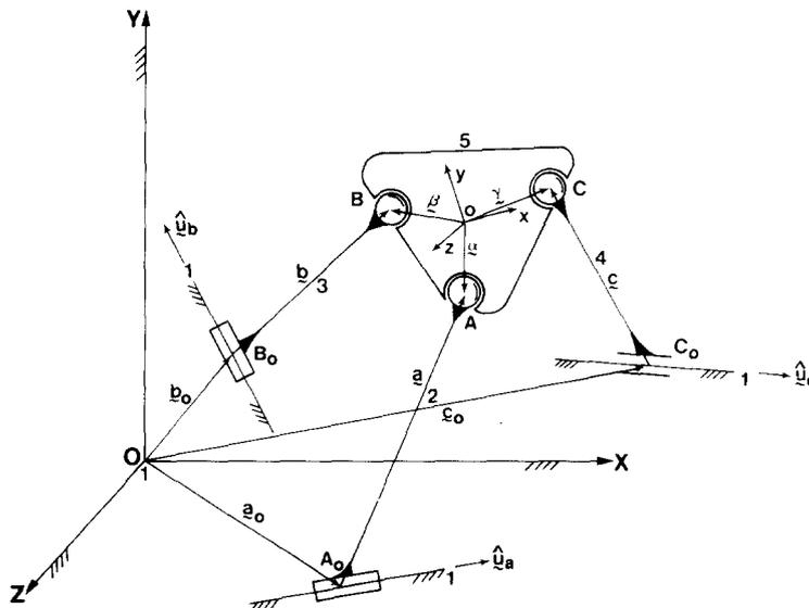
Fig. 1. Schematic drawing of the *RSSR-SC* mechanism and associated vectors.
