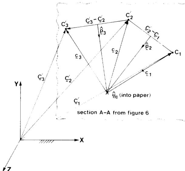
Fig. 7. Projections of the  $C-S$  link vectors onto the plane normal to  $\hat{u}_c$  and passing through point  $C_1$ .
