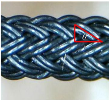
Fig 4: Braid angle measurement using microscope
