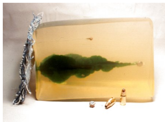
Figure 1: Snapshot of a cavity left in a ballistic gel by a bullet. Source: http://www.naaminis.com/pix/25gel02.jpg
