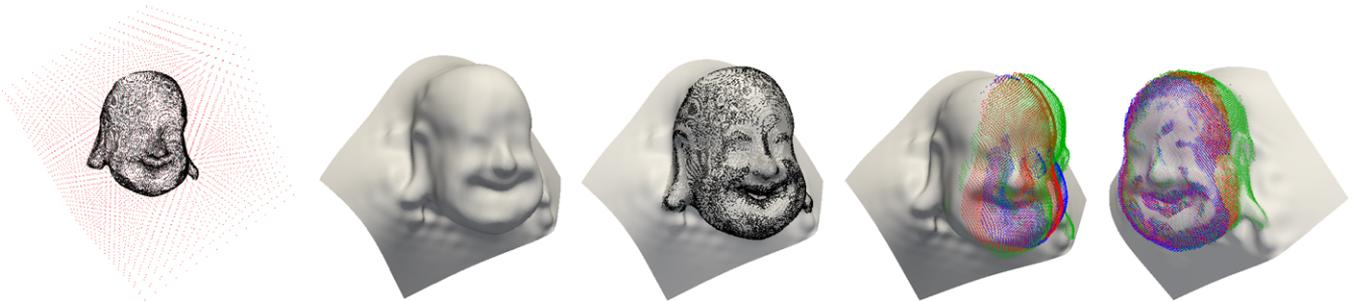
**(a)** Input point cloud (in black) immersed in a grid of nodes defining local max-ent shape functions. **(b)** Zero level set of the computed SSD function. **(c)** Comparison of the input point cloud and its implicit surface representation. **(d)** Implicit surface and partial scans for the Happy Buddha data set. **(e)** Registration of partial scans achieved using Algorithm 1.
